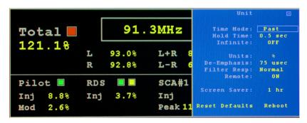
**Time Mode:** The Time Mode affects all the peak modulation readings and bar graphs. In Real Time Mode when a peak exceeds the current displayed peak the value is updated immediately to the new value and held for the Hold Time, until either a new peak is detected or the Hold Time is met. In Past Time Mode, the unit waits the Hold Time and displays the highest peak which was detected during that time period.
