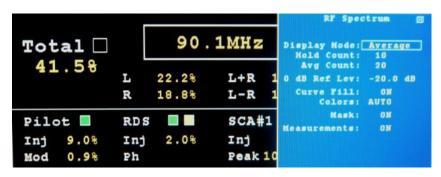
**Display Mode:** The Display Mode affects how the spectrum data is presented, in Realtime mode the spectrum is updated with new data each time, Peak Hold displays the highest value in the last Hold Count value of spectrums, Average displays the average of the last Average Count of spectrums, and Infinite holds the highest values until reset.
