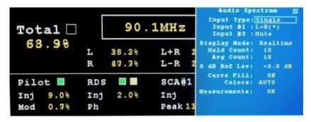
**Input Type:** Selects a single or dual input spectrum.
