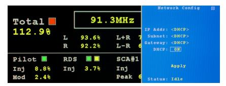
**IP Address:** DHCP must be disabled to enter a static IP **Subnet:** DHCP must be disabled to enter a Subnet **Gateway:** DHCP must be disabled to enter a Gateway
