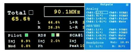
The **FMCS-1**provides 8 channels of analog audio output, 8 channels of AES/EBU output, and a headphone output. Any one of these output jacks maybe assigned any of the available audio: Mute, L, L(\*), R, R(\*), L+R, L+R(\*), L-R, L-R(\*), SCA#1, SCA#2, Pilot, Test 0dB, Test -3dB, & Test -6dB. The (\*) is the de-emphasized audio, otherwise the audio is flat. The SCA#1 & SCA#2 audio de-emphasis is selected in the SCA pop up window. The Test waveforms are a Test key sine wave at Test Test
