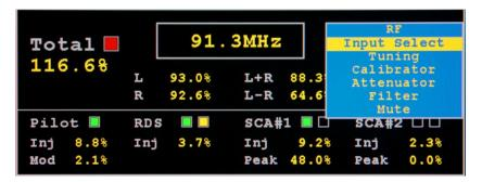
**Input Select:** Select which RF input is used Antenna (off the air) or High Level (tx site).
