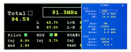
The FMCS-1 contains two independent SCA decoders SCA#1 and SCA#2. The parameters and setup of these decoders are the same so only one will be described.
