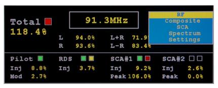
Many of the FMCS-1 Parameters and Information are accessed using popup menus. To access the popup menus press and hold down the encoder for 2 seconds. To navigate the popup menus rotate the encoder to highlight a menu choice and click the encoder. To exit the pop menu at any time, hold down the encoder for 2 seconds.
