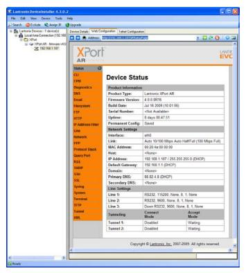
To set the Static IP 'CLICK' on the "Network" button on the left hand side. Next, 'SELECT' the "Configuration" box in the center. From this screen, ENTER the static IP address and subnet mask in the "IP Address" box using the format xxx.xxx.xxx xxxx.xxx xxx.xxx.xxx.xxx.
