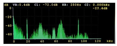
The Composite spectrum screen displays the Composite spectrum from 0 to 150 kHz. The amplitude and frequency scales are both adjustable and have cursors associated with them.
